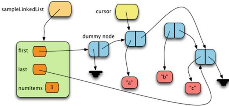
**Fig. 4.12** Deleting a Node from a Linked List
