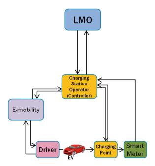
Fig. 2. Electrical vehicle charging SoS architecture
