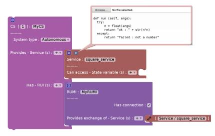
Fig. 28. Example of behaviour for a service
