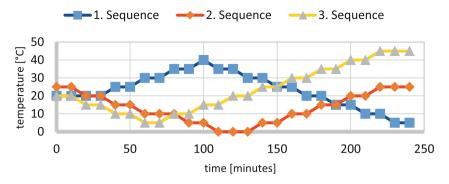
Fig. 6. Three test sequences of temperature set points.
