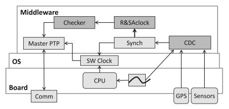
Fig. 1. Resilient Master Clock architecture.
