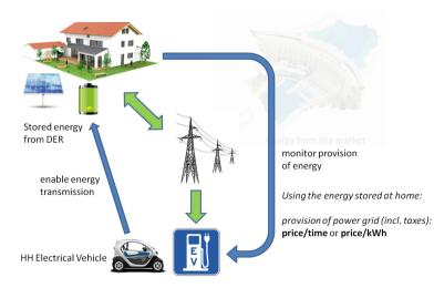
Fig. 27. The HH owner decide to recharge its EV with the energy stored at home
