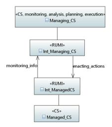
Fig. 2. Hierarchical control pattern
