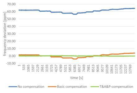
Fig. 8. Frequency deviation under different compensation models.
