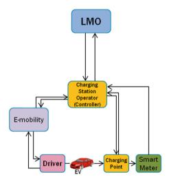
Fig. 13. Simplified functional diagram for an electrical vehicle charging station
