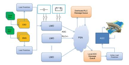
Fig. 30. Load measurement and predictive control architecture
