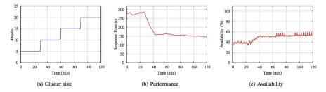
**Fig. 17.** Impact of cluster size on MapReduce performance and availability with #Clients = 10, #MC = 5
