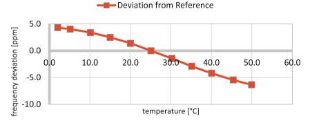
Fig. 4. Frequency deviation with respect to temperature.
