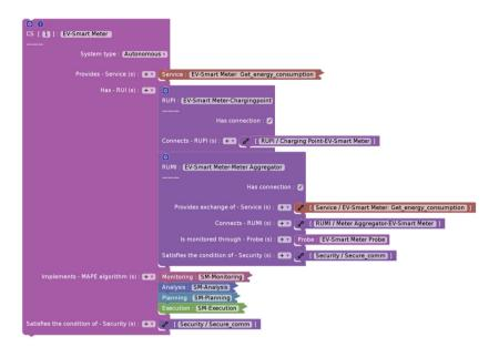
Fig. 10. The EV-smart meter CS Blockly model
