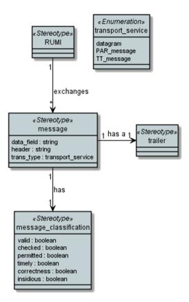
Fig. 11. An example subset of SysML meta-model to be transformed to Blockly
