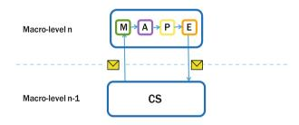
Fig. 4. Hierarchical control pattern
