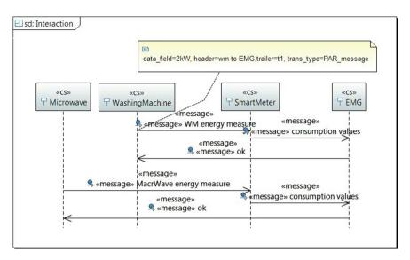
Fig. 14. Message exchange between CSs of a Smart Grid
