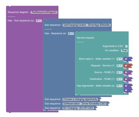
Fig. 30. Sequence diagram in supporting facility tool using Blockly
