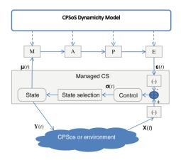
Fig. 12. Control and feedback parameters in MAPE-based control loops
