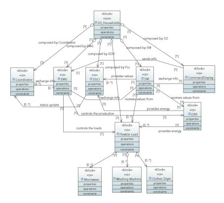
Fig. 13. Smart Grid household Block Definition Diagram
