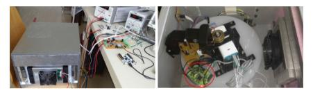
**Fig. 3.** Experimental chamber for obtaining training data for the compensation model. On the right the prototype of the CDC module has been highlighted with a red circle and is mounted on the rotating plate.
