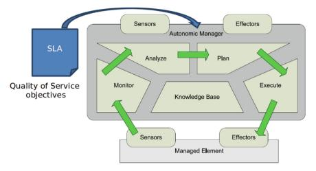
Fig. 1. MAPE control loop
