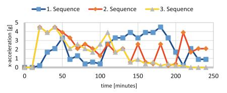
Fig. 7. Three test sequences of X-acceleration set points.
