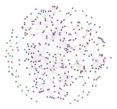
**Fig. 32.** The full SmartGrid model generated using the model query: "return true;" (i.e.: select all blocks). Here, the triangles represent systems, star represents the SoS and other blocks are represented by circles. The color of the blocks is the same as the one in the Blockly model.
